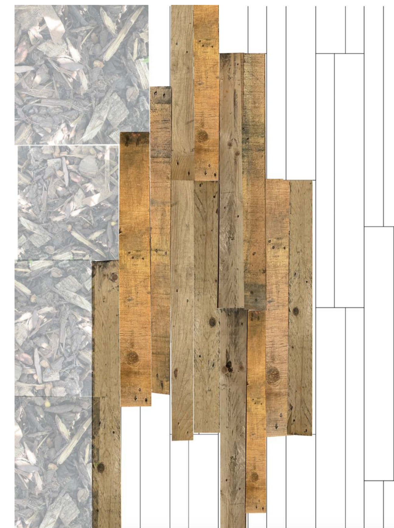
Floor made from recycled pallets, with bark and decomposing materials added to give effect of forest floor and the woody forest fragrance.
