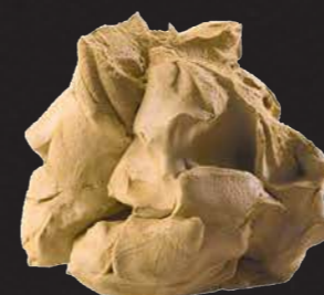
3 Mustard yellow +Iron Oxide, Fe 2 O 3 +Iron Hydroxide, FeO(OH)
