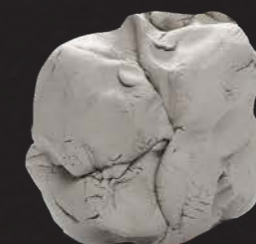
4 Light Grey +Silicon Dioxide, SiO 2 +Aluminum Oxide, Al 2 O 3 +Iron Oxide, Fe 2 O 3 +Carbon
