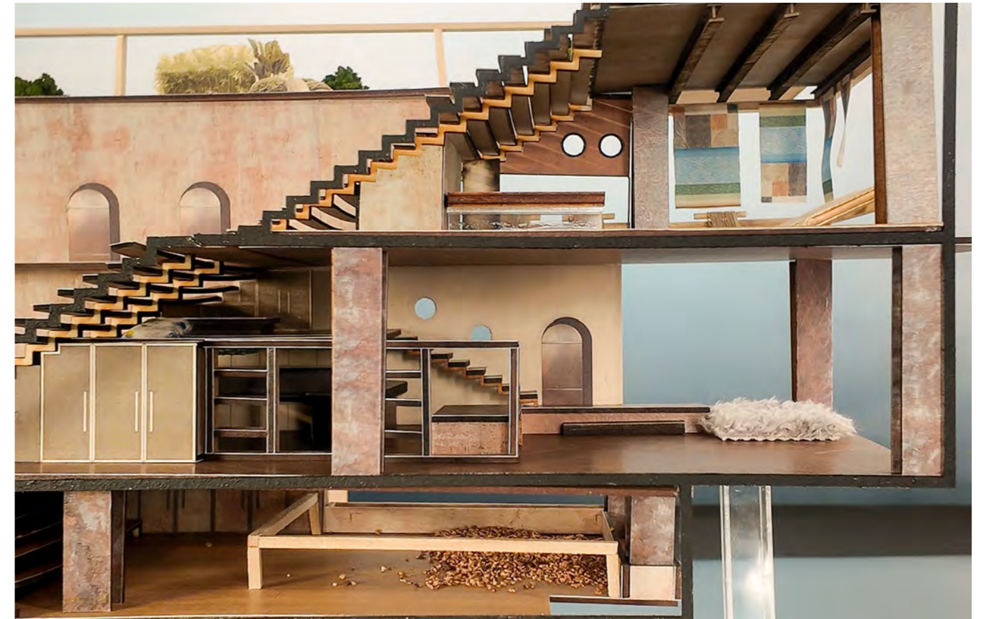
Right section where with spaces workshops in top, middle are living quarters and below are cow sheds. Adjences are such living quarters are accesible to both the spaces easily.
