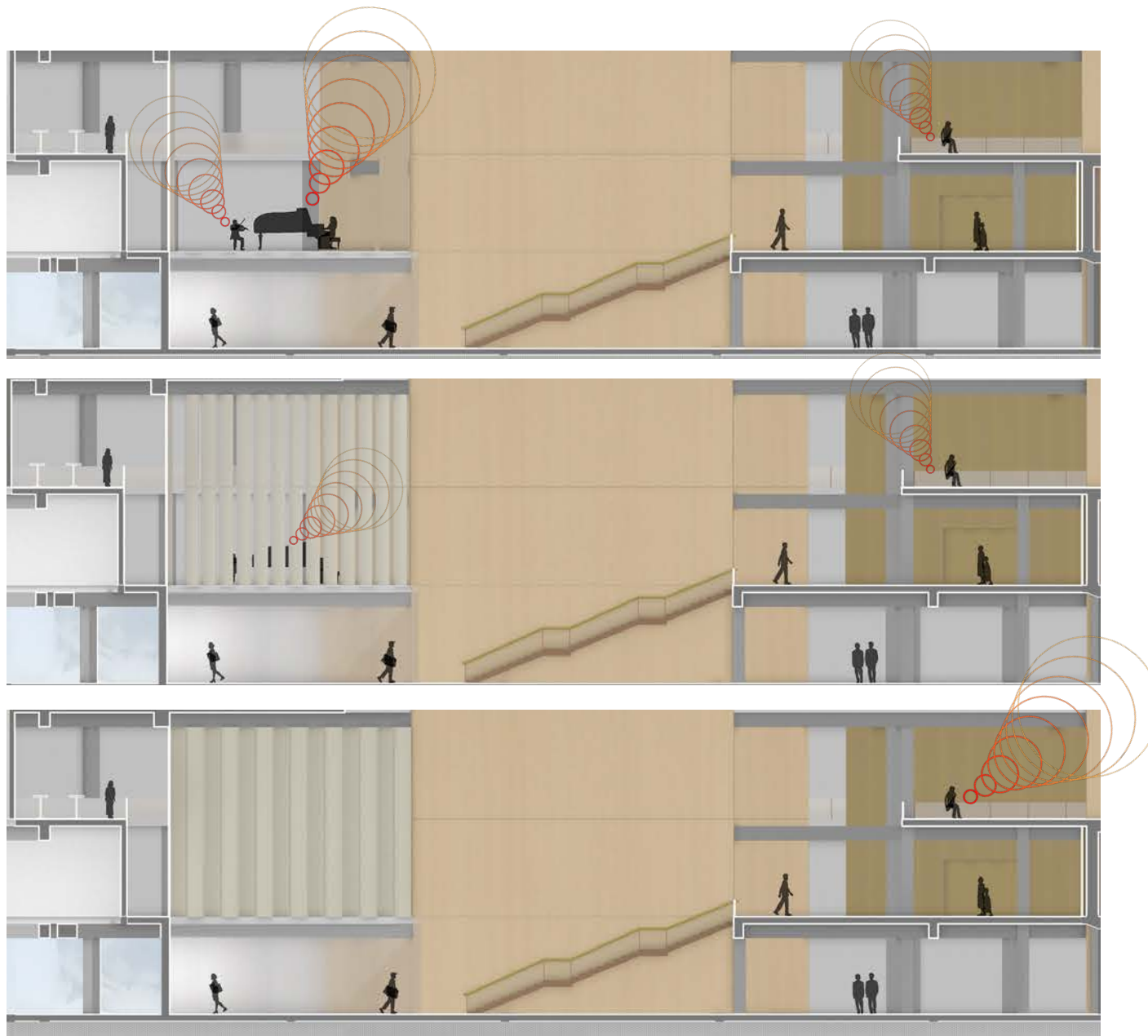
Movable acoustic panels connecting the public music area and the central staircase
