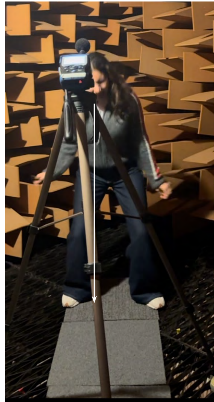
Scream aimed at acoustic wedges then measured with precision sound level
