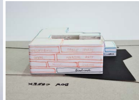
Option 1: MOVE and BUILDING activities are stacked vertically around the courtyard, the former relating to Bow Creek and the latter to Gillender Street.
